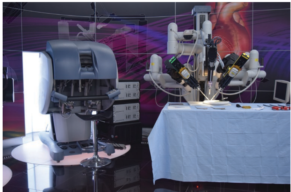
Fig. 1.9 The robot-assisted microsurgery system (courtesy of NASA/JPL-Caltech)
