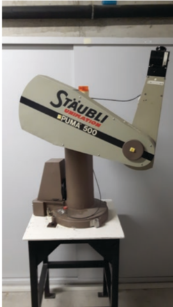
Fig. 1.3 The Puma 500 robotic arm (courtesy of Prof. Paolo Fiorini, University of Verona)
