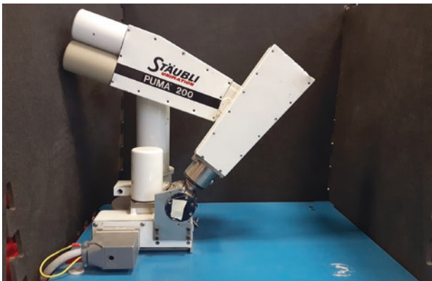
Fig. 1.4 The Puma 200 robotic arm (courtesy of Prof. Paolo Fiorini, University of Verona)
