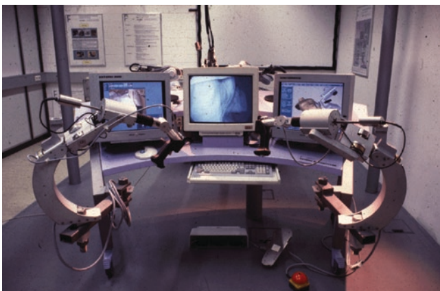
Fig. 1.7 The master station of the ARTEMIS surgical robot (courtesy of Prof. Alberto Arezzo, University of Torino)
