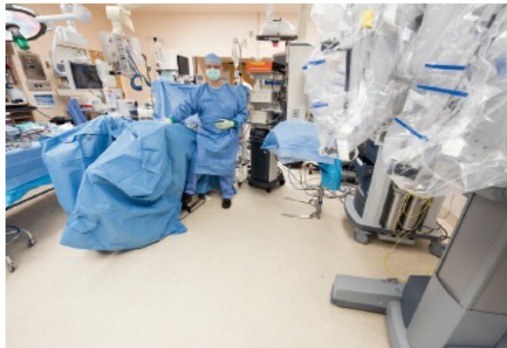
Figure 2.4. Demonstrates the 45-degree angle of approach for the patient cart toward the OR table. Surgeon directs the angle of approach. (Reprinted with permission, Cleveland Clinic Center for Medical Art & Photography © 2015 all rights reserved.)
