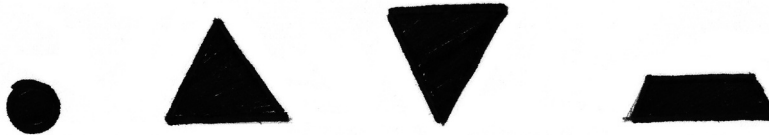
Fig. 2 Cut section of the needle tips. From left to right; taper (round), cutting, reverse cutting, spatulated
