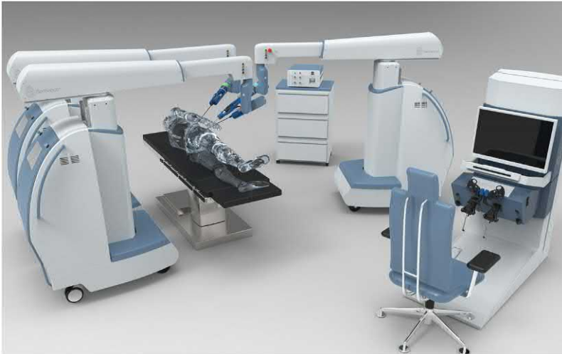
FIGURE 1.3 Typical Senhance three-arm setup for a patient in the lateral position. Credit: © 2018 TransEnterix, Inc.
