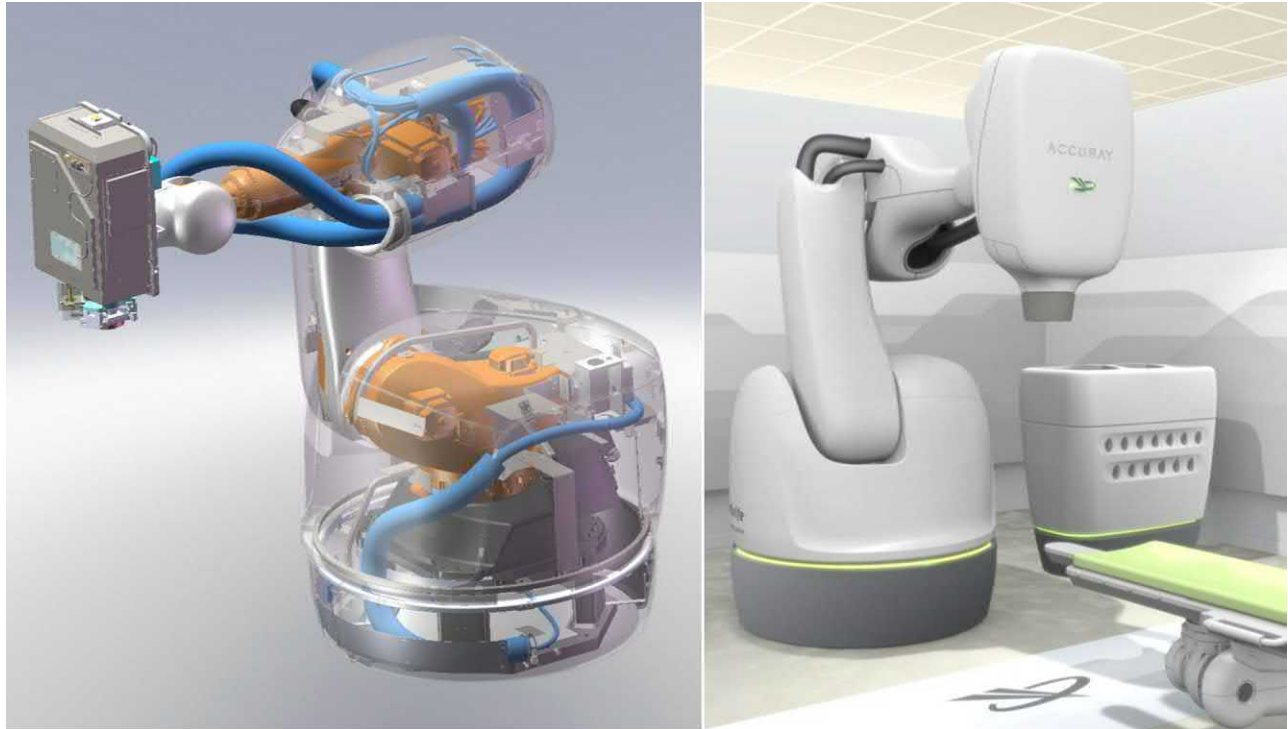
FIGURE 2.3 The treatment robot showing the KUKA robot, treatment head, cabling and tensioning mechanism, and pedestal (left), and in the treatment room with industrial covers fitted together with the treatment couch and Xchange table (right).
