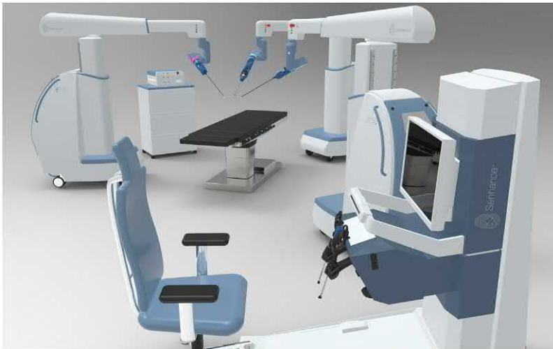
FIGURE 1.2 Typical Senhance setup that includes three manipulator arms for a supine patient. Credit: © 2018 TransEnterix, Inc.
