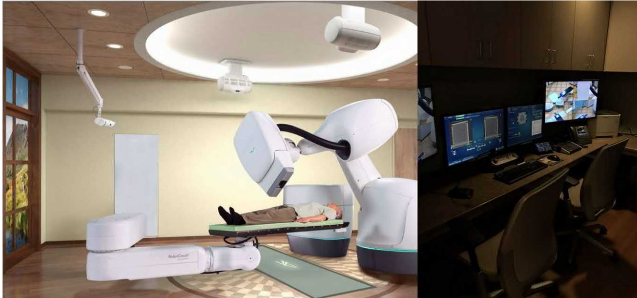
FIGURE 2.1 The CyberKnife treatment suite. The left image shows the patient lying on a flat couch mounted on a robotic manipulator, with the linear accelerator mounted on a second robotic manipulator at the head of the couch. In this case the multileaf collimator assembly is shown attached to the treatment robot. Behind the patient and treatment robot in this image is the pedestal used to store the three alternative secondary collimator assemblies when not attached to the treatment robot. The two ceiling-mounted X-ray tubes are shown, with the floor-mounted X-ray image detectors housed under the rectangular green panel beneath the couch. The optical camera array in its ceiling-mounted boom-arm is shown near the left side of the image. The right image shows the control area. The treatment delivery computer to the left displays live X-ray images, DRRs, tracking results, and treatment-related data during treatment. To the right, the CCTV and intercom systems monitor and communicate with the patient during treatment. The small white console next to the keyboard contains low-level controls to initiate and interrupt treatment. DRR , Digitally reconstructed radiograph. Control area image courtesy Dr. J.A. Gersh, Gibbs Cancer Center and Research Institute—Pelham, Greer, SC, United States.
