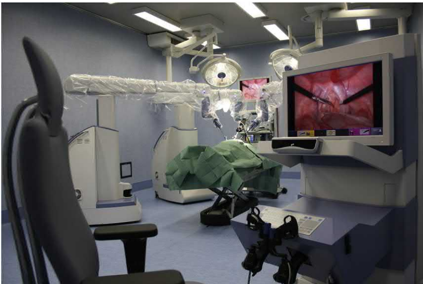
FIGURE 1.1 Typical operating room setup with the Senhance Surgical System. The console is in the foreground with the patient table in the middle of the image with the manipulator arms, laparoscope, and instruments in place. A secondary monitor, which shows the same view of the operative field that the surgeon sees, is available to the assistant and nurse.
