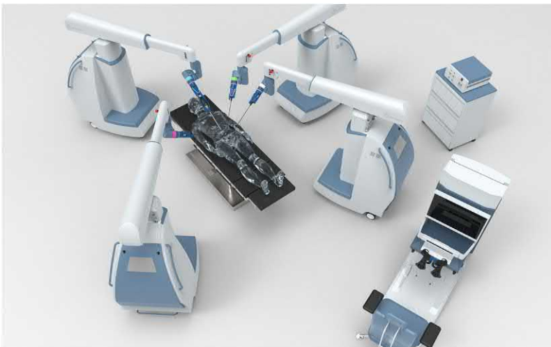
FIGURE 1.4 Senhance four-arm setup for a supine patient. Credit: © 2018 TransEnterix, Inc.
