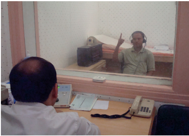
Figure 4.2. Two-room audiometry setup. Audiometrician watches responses of the patient sitting across a glass partition.
