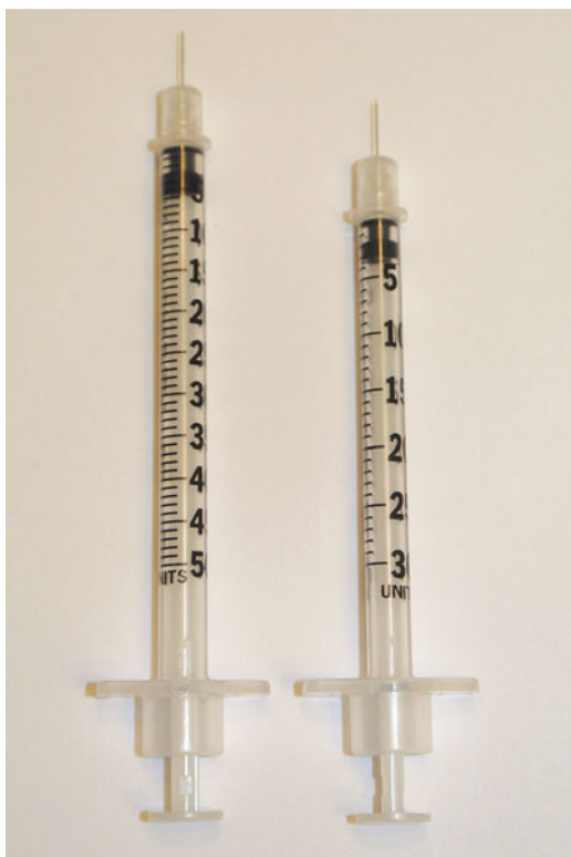
Fig. 3.1 Dripless 0.5 mL (left) and 0.3 mL (right) BD insulin syringes may be used for BoNTA injections. These syringes have a pre-attached 31-gauge needle.
