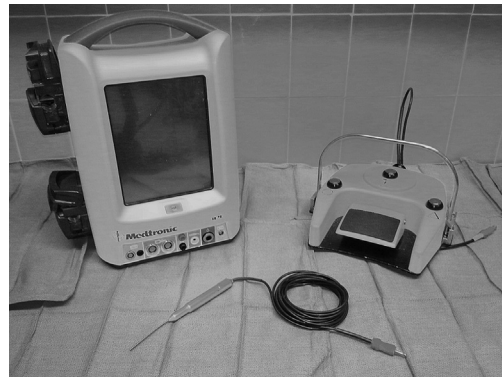
Figure 1-5 Medtronic Skeeter microdrill for footplate work.
