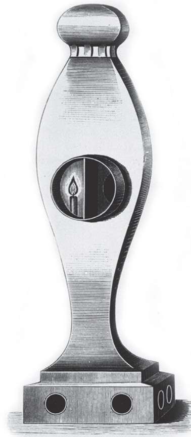
Fig. 1.4: The endoscopic light source developed by German physician Philip Bozzini involved candle light reflected by a mirror into the endoscope.
