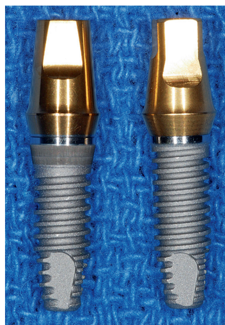
FIGURE 2-6. An implant body (gray color) is usually separate from the implant abutment (gold color). They are most often connected together with an abutment screw. (Left, internal hex BioHorizons Dental Implants; right, external hex BioHorizons Dental Implants, Birmingham, AL).
