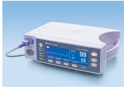
FIG. 1-21 Nellcor OxiMax N-600x pulse oximeter. (Courtesy Nellcor Puritan Bennett, Boulder, CO; now part of Covidien.)
