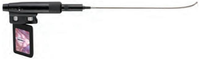
**Fig. 1.16.** The Clarus Video System incorporates a curved stylet containing a CMOS chip video camera surrounding by a malleable but rigid protective metal sheath. Images are displayed on a video screen attached to the handle. The screen can swivel for optimal viewing as the stylet is inserted into the mouth. (Courtesy Clarus Medical, Minneapolis.)
