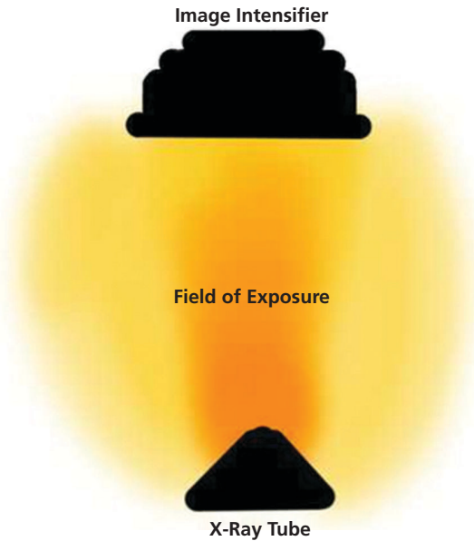
Figure 1.3 Field of radiation around the fluoroscopy machine. The emitter is at the bottom, and the image intensifier at the top.
