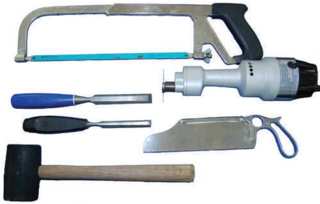
Fig. 1.8 Handsaws (long and short) for bone; electric Stryker bone saw; chisel (broad and narrow blades); rubber mallet.
